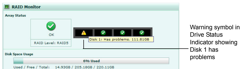
Figure 4: RAID Monitor displaying a failed disk
