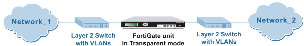
Figure 8: Example layer-2 switch network
