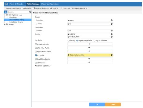
Note: In case the FortiGate has multiple interfaces connected to Internet, configure the interface policy for all such Internet-facing interfaces.
